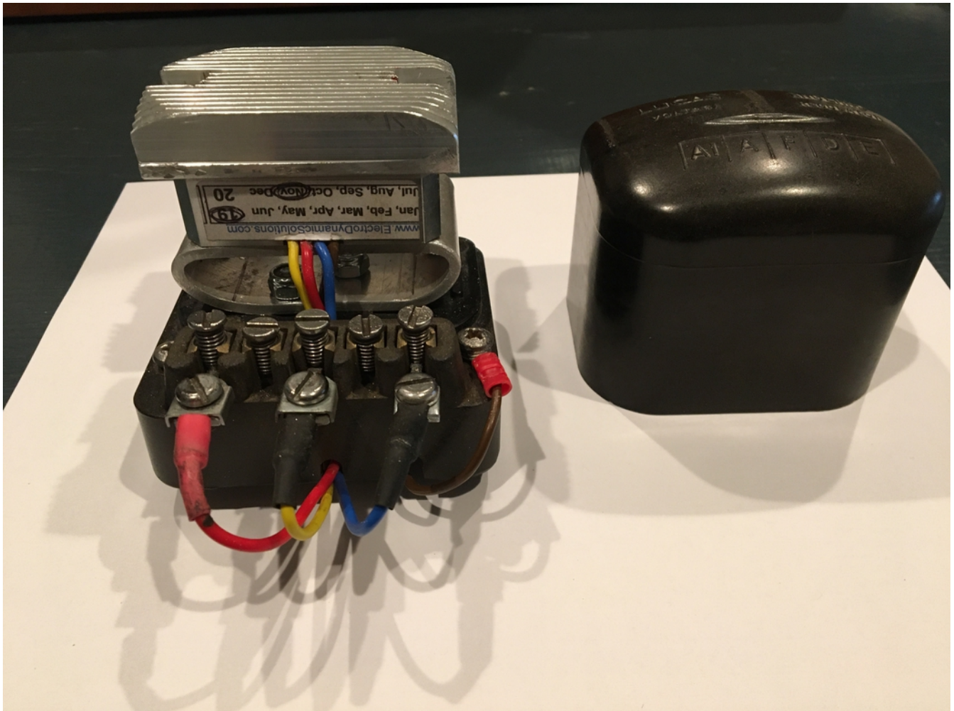
Typical installation of a DVR3 into the existing housing
