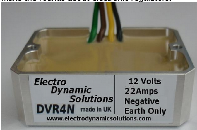
DVR4 Electronics cut out, voltage and current regulator
